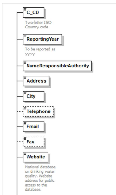
Figure 6.1. Both the element Telephone and Fax is optional information to report – this indicated with a dashed line around the defined element.
